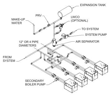
FIG. 37 Primary/Secondary Piping of Multiple Boilers
